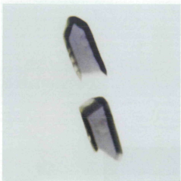
Fig. 2. Photograph of DAO crystals of the purple intermediate (see text for the method of preparation). Approximate dimensions of the crystals: 1 \times 0.4 \times 0.2 mm.
